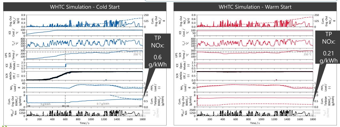
The ICE with future technology can stay below the 0.46 g/kWh NOx emission limit in WHTC – Weighted Tailpipe NOx emissions: 0.265 g/kWh 12-06-2023
